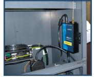
Each wireless client is programmed with a unique IP Address which ensures that a CNC program cannot be sent to the wrong machine. It also means that all machines can load programs at the same time.
